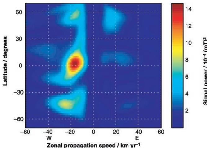
**Fig. 3.** Power moving with eastward zonal speeds between  $-60$  and  $60 \text{ km year}^{-1}$  in time-longitude diagrams of the residual field, every 2° latitude from 70°N to 70°S. A maximum is found at the equator, indicating a robust measurement of westward motion (at  $-17 \text{ km year}^{-1}$ ) in this region. Weaker signals are observed at mid-latitudes, particularly near 40°S ( $-26 \text{ km year}^{-1}$ ) and 55°N ( $-18 \text{ km year}^{-1}$ ).
